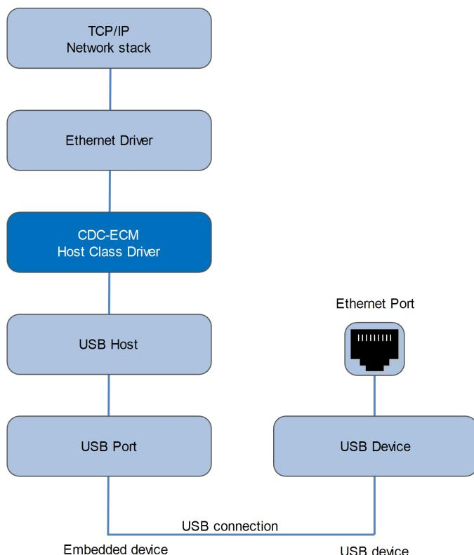
The host implementation allows the host system to transfer Ethernet packets to/from a remote Ethernet port at the other end of the USB connection. It connects to a USB device that has an Ethernet port on it that connects to a real or virtual network.
