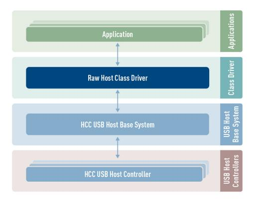
The lower layer interface is designed to use HCC Embedded's USB Host Interface Layer. This layer is standard over different host controller implementations; this means that the code is unchanged, whichever HCC USB host controller it is interfaced to. For detailed information about this layer, refer to the <u>HCC USB Host Base System User Guide</u> that is shipped with the base system.
